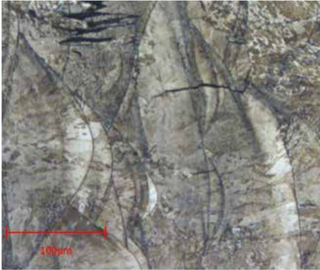
Fig. 8: Contrasted specimen. The welded-based microstructure of the manufactured workpiece is clearly visible.
