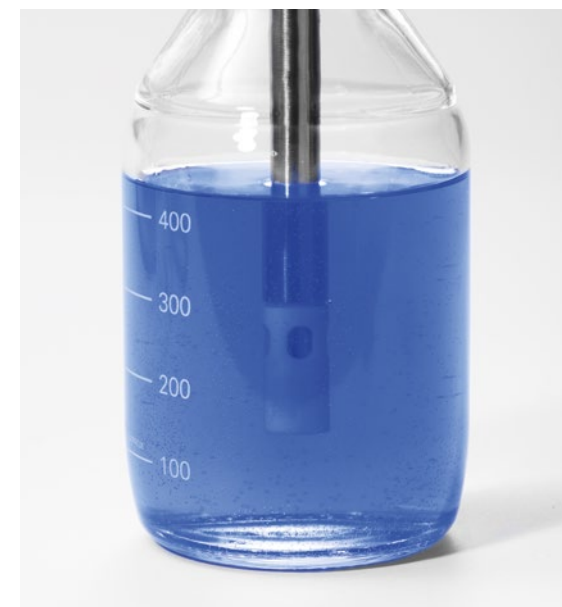
Measurement using the FLOWGUARD in a vessel
